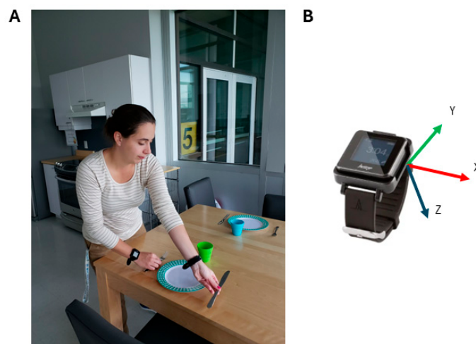
Figure 2. Experimental setup for the accelerometry assessment. (A). Participant wearing one accelerometer at each wrist while setting the table. (B). Accelerometer used for the assessment including a representation of the x -, y -, and z -axes.
